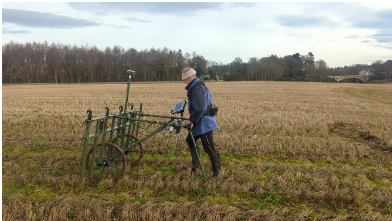
Figure 24: Simon Payne using the SENSYS magnetic gradiometer. Photo Simon Allerton.
